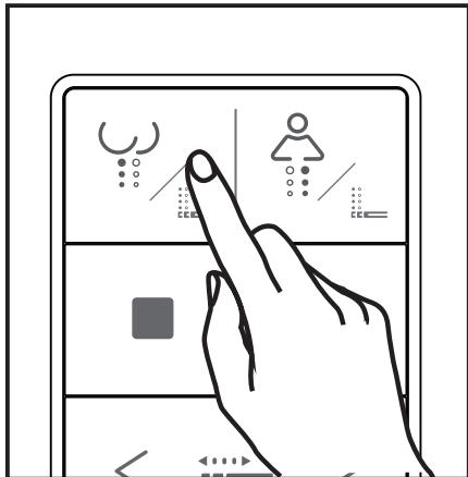
When the Rear wash or Lady wash is activated, press the "Rear wash or Lady wash" key again to activate the mobile cleaning under this function, and the nozzle will move back and forth.
