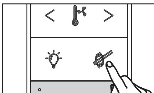
2. Press the Nozzle Cleaning button. The nozzle extends without water, and the main unit makes a short beep every 3 seconds during the cleaning process.
