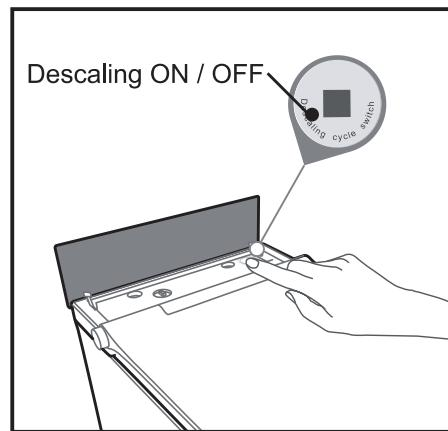
2. Press the descaling button and start the water tank drainage, the nozzle will self-clean during the drainage process, accompanied by drops beep. If misoperation, the product can be used normally after power off and restart.
