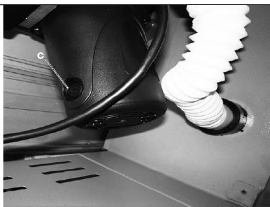
Check the carbon brushes after the first 50 hours of operation with a new machine or when new brushes are fitted. After carrying out the first check, repeat the check every 10 hours of operation.
