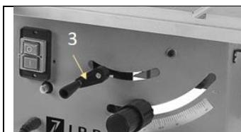
The saw blade can be raised and lowered by the crank (3). If the crank is turned clockwise, the saw blade is lowered. Counterclockwise it is raised
