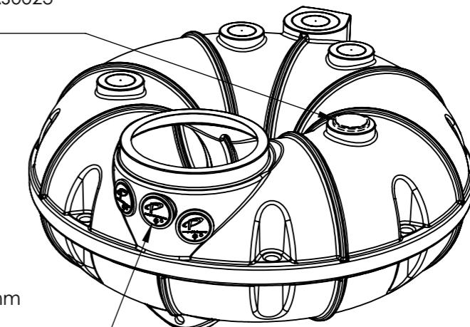
3 x Bohrung Ø127mm
