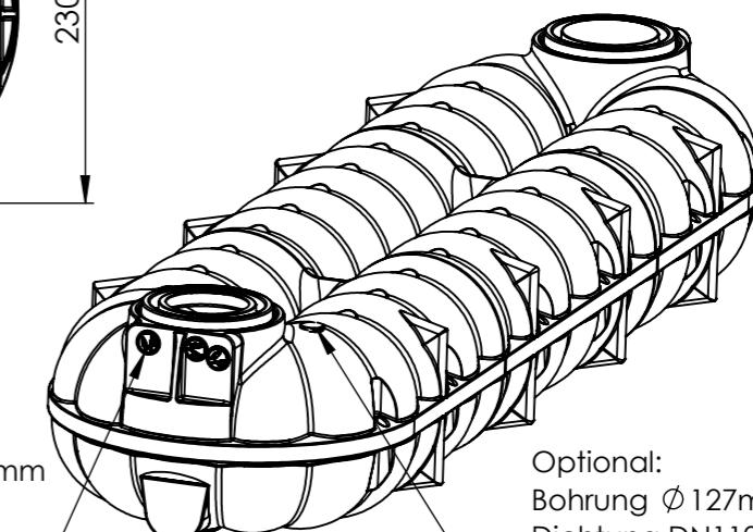
3 x Bohrung Ø127mm
