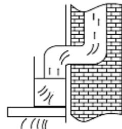
**Horizontally:** Install the exhaust hose to an exhaust outlet equipped with an air grille\*.
