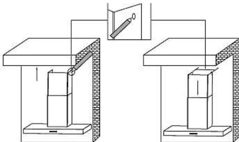
10. Drill two  $\varnothing$  8 mm holes for the fixing bracket in the appropriate height. Install the fixing bracket on the corresponding position on the wall (s. fig. below).
