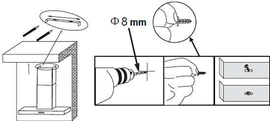
11. Attach the **outer** chimney by fixing it at both sides (s. fig. A).
