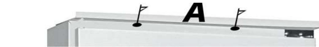
Fixing points to fix the appliance with the assembled components A+B and the supplied woodscrews in the cabinet.
